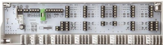
**Basic+ terminal blocks** provide power for all control elements. Available with heating - cooling version with possibility to control 6 or 10 heating zones. Both versions are available in 230V and 24V version (required 230/24 V AC transformer). Terminal blocks can control the boiler and circulation pump operation. In addition the automatic mode can be set to work with Normally Closed or Normally Open devices.
