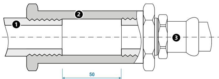
Principle of connecting KAN-therm Inox elements with zinc-plated steel
