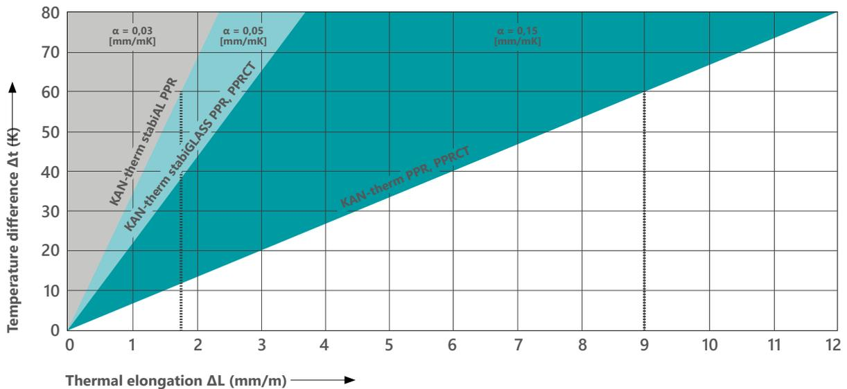
Comparison of the thermal expansion factor in uniform PPR or PPRCT and both stabiAL PPR and stabiGLASS PPR and PPRCT pipes.
