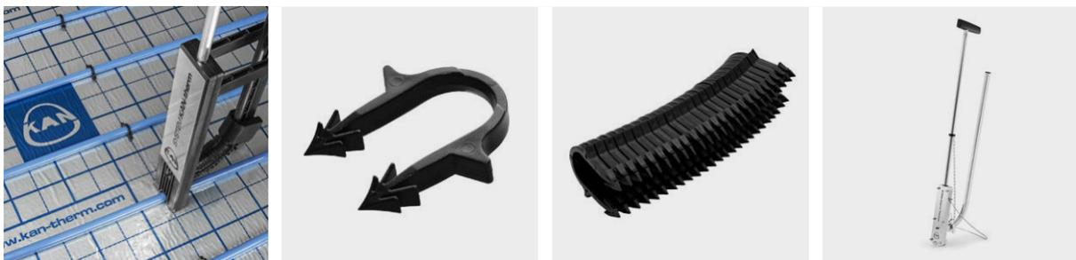
Pipes are fixed to Tacker panels with clips driven with a Tacker tool. For 20 mm thick styrofoam panels use short clips driven with a Tacker tool for short clips. Thanks to an overprinted grid it is easy to lay pipes at a determined spacing. You can use Ø14×2, 16×2, 16×2,2, 18×2, 20×2, 20×2,8 mm pipes spaced every 10-30 cm.
