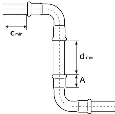
A – Pipe insertion depth in the fitting,
