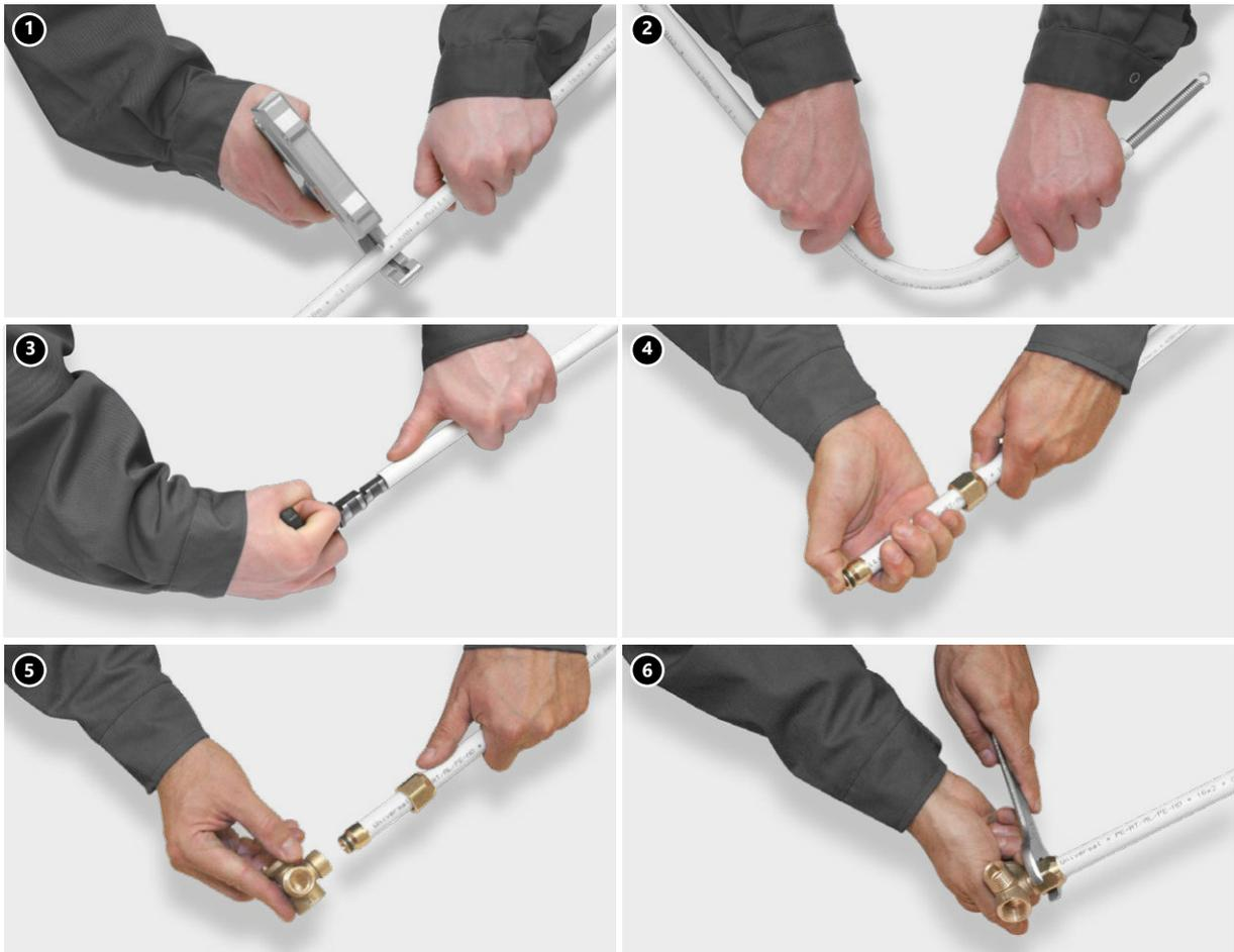
1. Using a pipe cutter for PERTAL pipes or a pipe roller cutter, cut the pipe perpendicularly to its axis at the required length.
