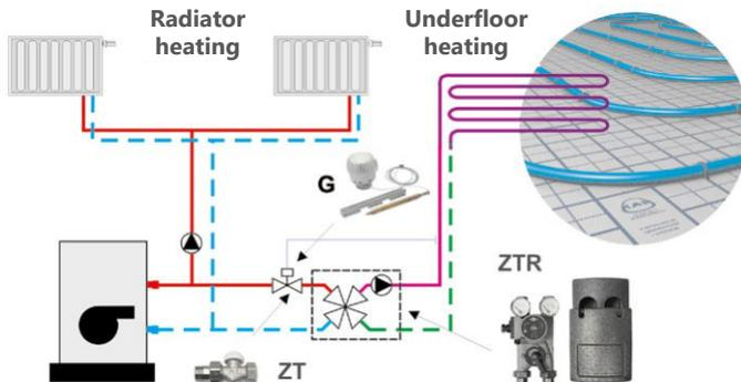
A KAN Bloc (ZTR) mixer with a 4-way valve provided additionally with a thermostatic valve (ZT), adjusts a system semi-automatically.
