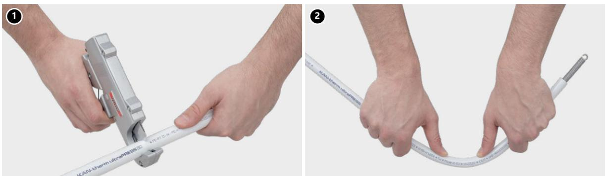
1. Using a pipe cutter for PERTAL pipes or a pipe roller cutter, cut the pipe perpendicularly to its axis at the required length.
