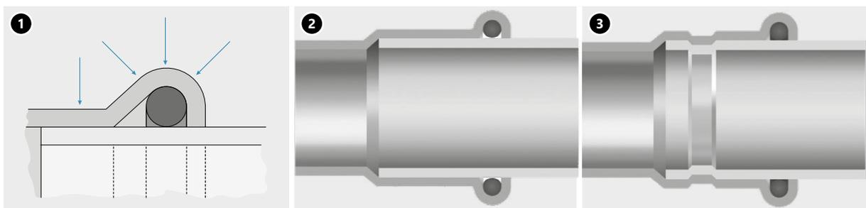
1. Pressure directions in a "Press" joint
