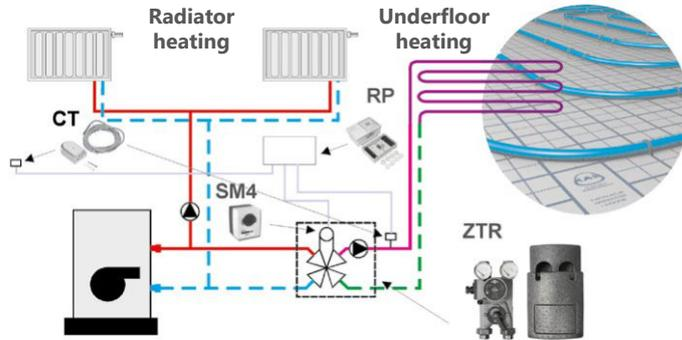
A KAN Bloc (ZTR) mixer provided additionally with an servomotor, weather regulator (RP) and temperature sensors adjusts the system automatically, e.g. as a function of the external temperature.
