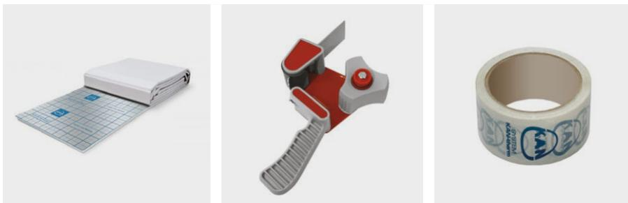
Use panels Tacker EPS 100 038 (PS20) for standard floor slab loads up to 30 kN/m<sup>2</sup> in residential or office buildings. The foil glued onto plates serves as a damp proof insulation to DIN 18560 and can be overlapped, thus panels can be laid tight. To seal places, where plates join, use adhesive tape dispensed from a hand feeder.
