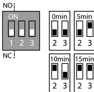
The operation mode setting is carried out using Jumper 1:
