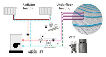
A KAN Bloc (ZTR) mixer with a 4-way valve provided additionally with a thermostatic valve (ZT), adjusts a system semi-automatically.
