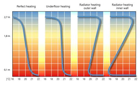
Vertical distribution of temperature for various types of heating
