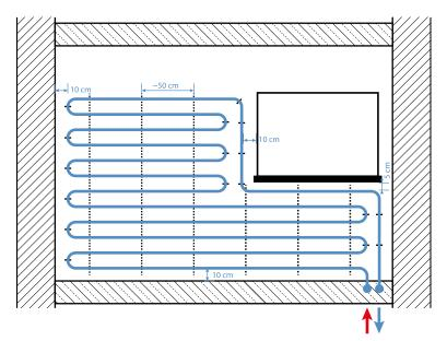
Mounting distances in wall heating/cooling
