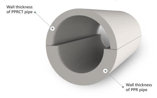
PPR and PPRCT pipe with equivalent pressure rating
