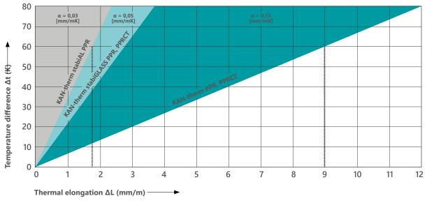
Comparison of the thermal expansion factor in uniform PPR or PPRCT and both stabiAL PPR and stabiGLASS PPR and PPRCT pipes.
