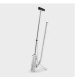
Pipes are fixed to Tacker panels with clips driven with a Tacker tool. For 20 mm thick styrofoam panels use short clips driven with a Tacker tool for short clips. Thanks to an overprinted grid it is easy to lay pipes at a determined spacing. You can use  $\emptyset$ 14×2, 16×2, 16×2, 18×2, 20×2, 20×2,8 mm pipes spaced every 10-30 cm.
