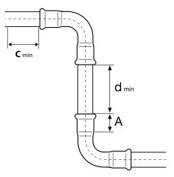
$\begin{array}{lll} {\rm A\,-} & {\rm Pipe~insertion~depth~in~the~fitting,} \\ {\rm d_{min}\,-} & {\rm minimum~distance~between~fittings} \\ {\rm allowing~press~correctness} \\ {\rm C_{min}\,-} & {\rm minimal~distance~of~fitting~from~wall} \end{array}$
