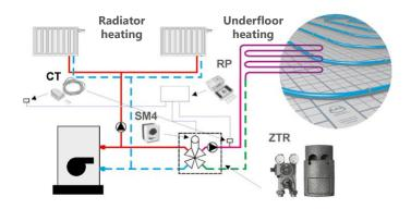
A KAN Bloc (ZTR) mixer provided additionally with an servomotor, weather regulator (RP) and temperature sensors adjusts the system automatically, e.g. as a function of the external temperature.
