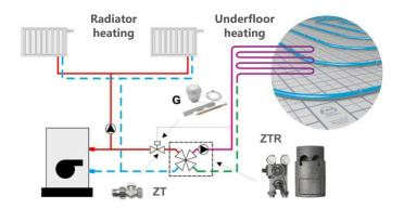
InoxFlow USVP and USFP series manifold connected directly to a heating system operates as a local mixing system. A thermostatic head with a capillary tube serves as a protection against a possible temperature rise. It can be adjusted "down" from 55°C.
