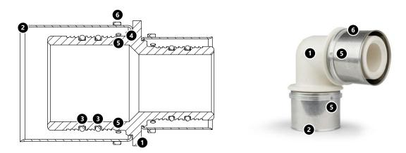
View and cross-section of KAN-therm ultraPRESS fitting without a colored ring.
