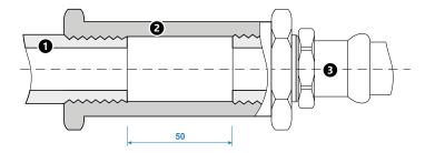
Principle of connecting KAN-therm Inox elements with zinc-plated steel
