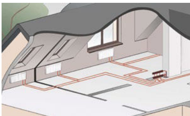
Manifold – tee system in a heating installation
