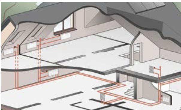
“Vertical” system in a heating installation
